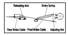
To check this, lay the open Evacu-Trac on its side. Locate the Front Brake Cable. It should have approximately 19 mm (3/4 in) of slack, when measured vertically from the reference point shown in the drawing to the right.
