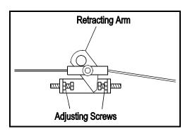
3. The final step is to ensure that the Track Parking Brake is functioning correctly. It is designed to stop and hold rated load on the stairway. To do this, the Brake Spring must pull on the Brake Mechanism without any resistance from the Brake Cable. This can happen if the Front Brake Cable does not have sufficient slack.
