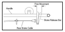
When you squeeze the Brake Release Bar it should travel until it just makes contact with the lime green Handle. This will allow you to comfortably hold Brake Release Bar in its released position when pushing Evacu-Trac on flat surfaces or descending a stairway.
